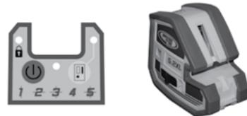
1. Unlock the laser's compensator by sliding the switch to the LEFT.
